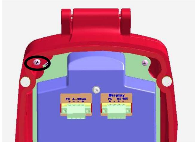
Figure 34 Internal Ground Terminal
