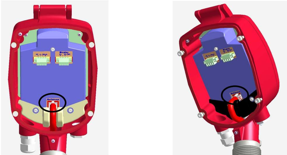
Figure 16 Connect the Cable Connect to the Electronic Card
